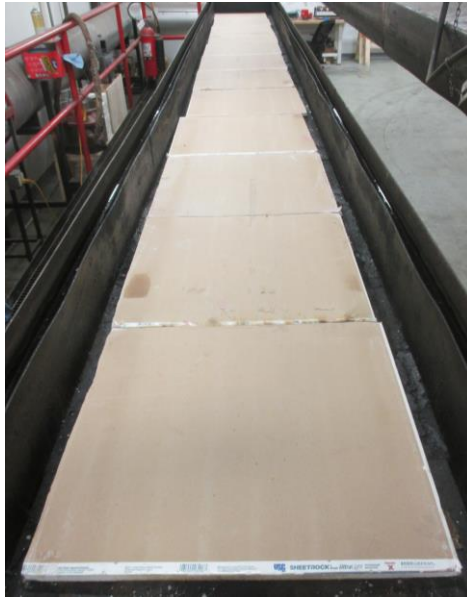
Photo No. 3 Unexposed Surface of the Test Specimen (Post-test)
